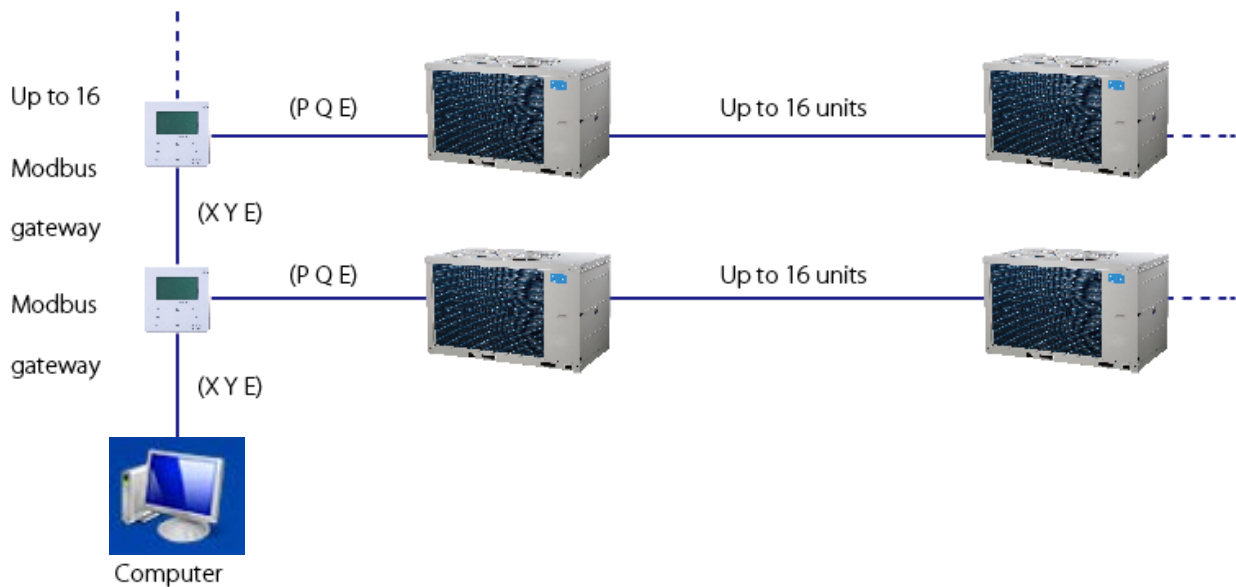
Figure 3-4.5: Modbus Gateway wiring connection
