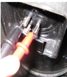
Figure 4-4.4: Measuring resistances among compressor terminals
