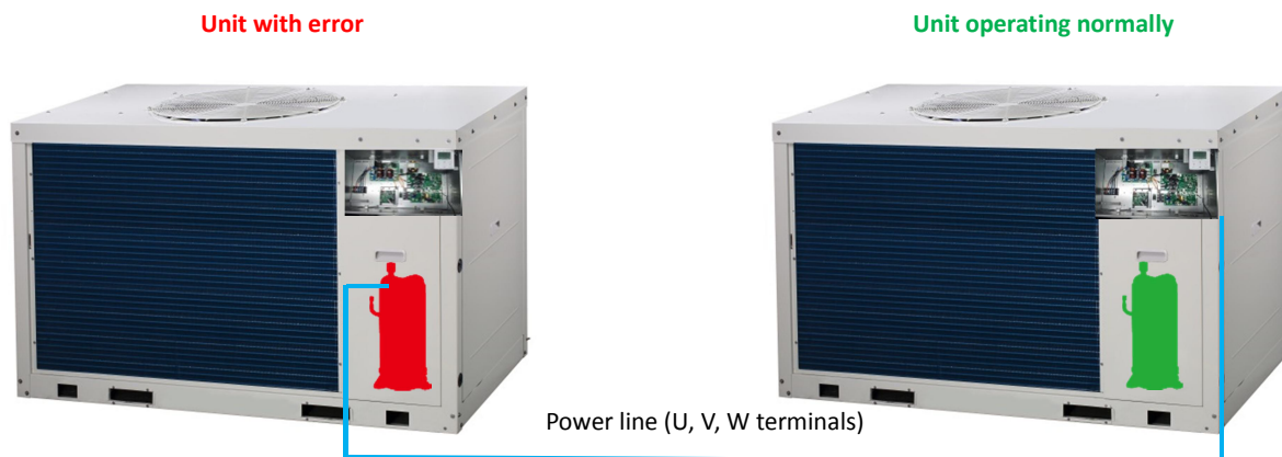
Figure 4-4.10: Connecting compressor to an error-free unit
