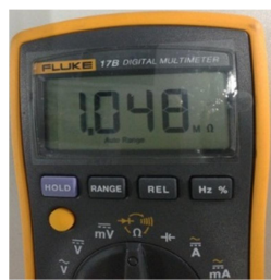
Figure 4-4.4: Measuring resistances among compressor terminals
